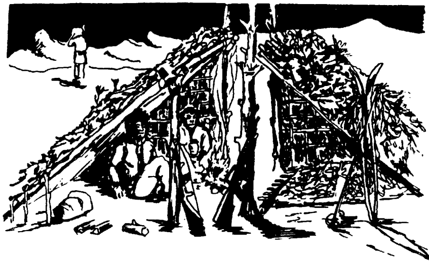
Figure A-2. The Double Lean-To Shelter.
